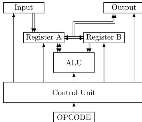
The control unit shall generate the control signals represented in the diagram by single arrows according to the operations given in the table. The operations are defined by a 3 bit number, the operation code:
