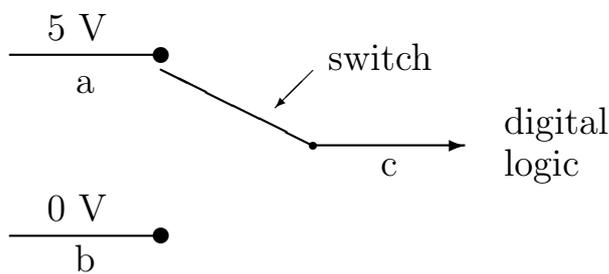
The SPDT switch connects either of the terminals a or b to the common terminal c. When the switch is flipped from one position to another, the springy metal switch might bounce off from the contact thus giving rise to a chattered signal on terminal c. This is referred to as chatter or **contact bounce**. A digital logic connected to c will see the chatter and detect it as multiple on-offs despite the switch was flipped only once.
